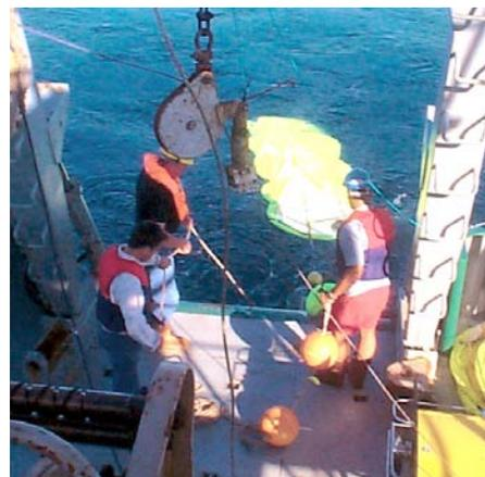
Drifters like this one, with an orange surface marker and a large 'sock' beneath, are tracked by satellite to map water movements.
