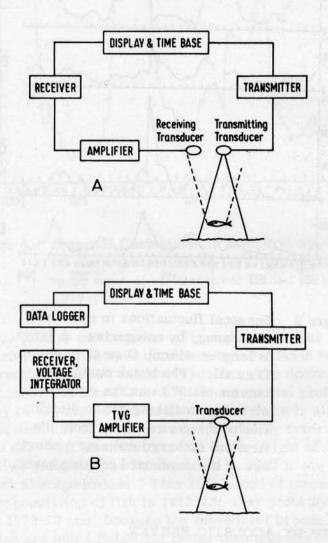
Figure 10 (A) Simplified diagram of the echo-sounder system fitted to most fishing boats.
