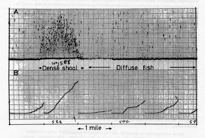
Figure 11 Record of echo signal strength made on an acoustic survey.
