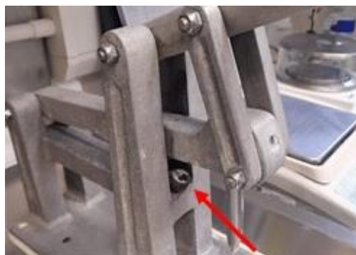
Figure 3: Opening a gastropod using an oyster cracker
