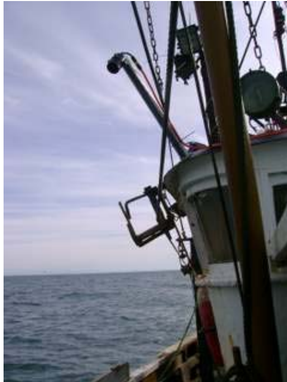
Figure 2. View of the third camera (3.6 mm lens), located to observe the codend as it was hauled on board, to monitor possible slippage, to quantify the total catch, and to monitor the starboard warp to interpret fishing activity. The camera was mounted on a 600 mm extension arm to give greater coverage and to ensure that the camera was clear of lifting rigging.
