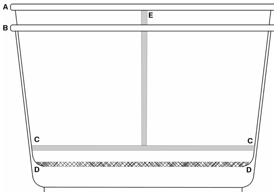
Figure A 1.1 The experimental fish-tank showing outer normal tank (B), inner tank (A) with a stainless steel mesh bottom(D). The perspex cover (C) and tank divider (E) were removed during breeding (lay opportunities) so that eggs could fall through the mesh.
