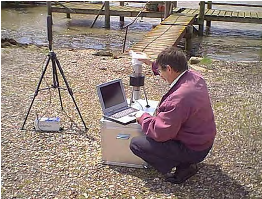
Figure 1: Operation of the NaI System in the field.
