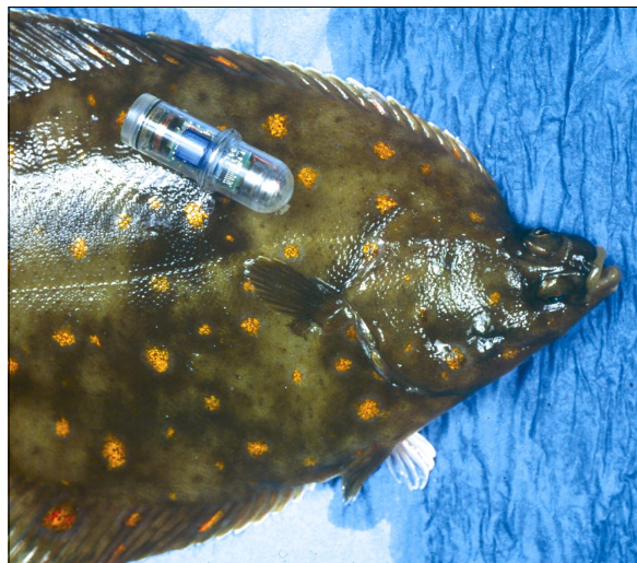
Figure 2. Data storage tags permit the detailed behaviour of many individual fish to be recorded at the same time over long periods. The tags must be recovered through a fishery.
