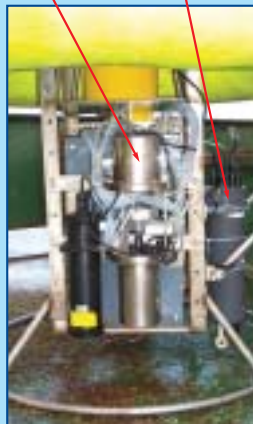
Figure 2: SmartBuoy - a view of the subsurface instrument payload with NAS2E in-situ nutrient analyser and Aqua Monitor.
