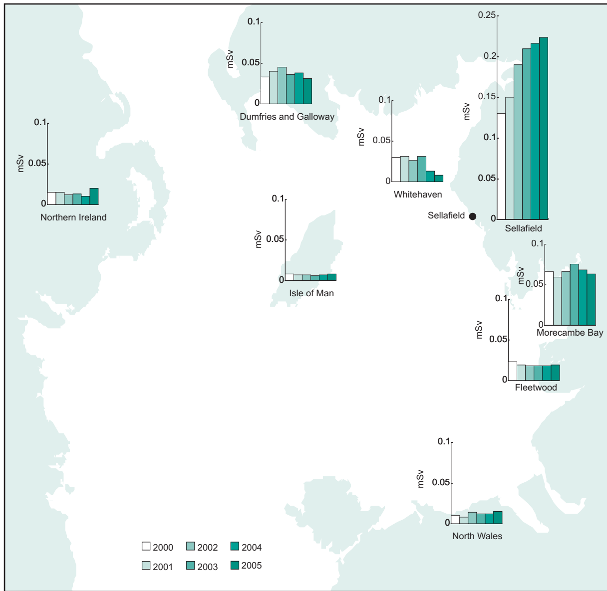
Figure 3.22 Individual radiation exposures to seafood consumers from artificial radionuclides in the Irish Sea, 2000-2005
