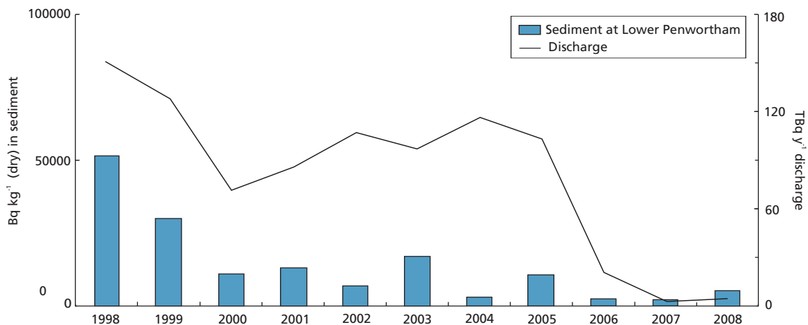
Figure 2.3. Total beta in liquid discharges from Springfields and concentrations in sediment at Lower Penwortham, 1998-2008
