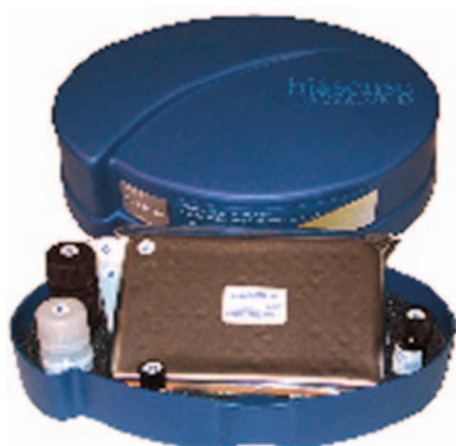
Figure 1. The ASP ELISA kit contains a sealed pre-coated 96-microwell plate, and all the key components required to accurately measure DA levels in 36 individual samples
