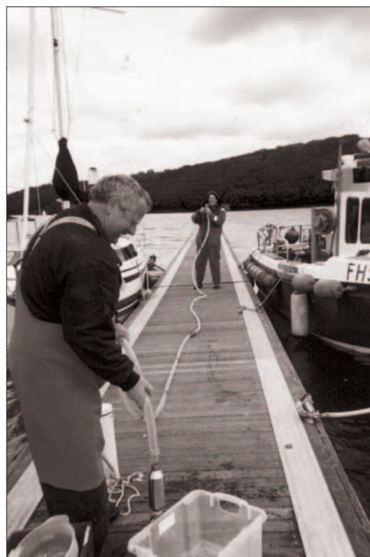
Figure 1. Use of 15 m (three 5 m sections) tube sampler in the Fal
