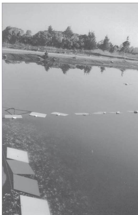
One of the ponds showing 4 tiles in the foreground against the pond edge, and then the beginning of a row of tiles leading into the pond centre, comparing settlement at different locations. The polystyrene was effective at keeping the tile angles approximately constant in the centre and along the pond edge. This picture also shows the mussel shell on the pond edge
