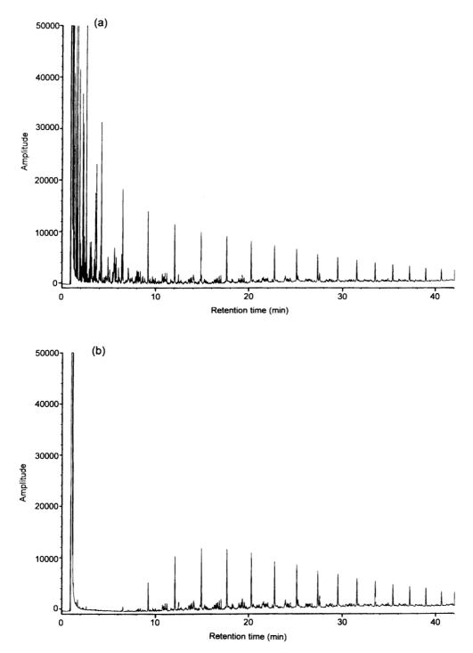
Figure 1. Gas chromatographs showing spectra of whole (a) and weathered (b) Kuwait crude oil
