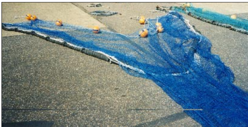
Figure 3. High-headline bass trawl, showing headline with floats and rubber bobbins on the footrope
