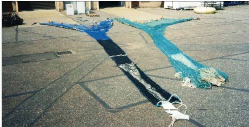
Figure 2. Two high-headline bass survey trawls, made to the same specification, but constructed with different coloured yarns
