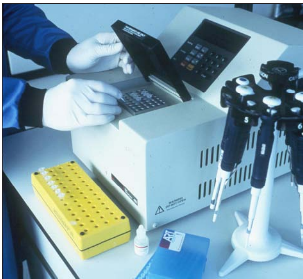
Figure 30. Isan automatic thermal cycler used for Polymerase Chain Reaction PCR - for amplification of DNA.
