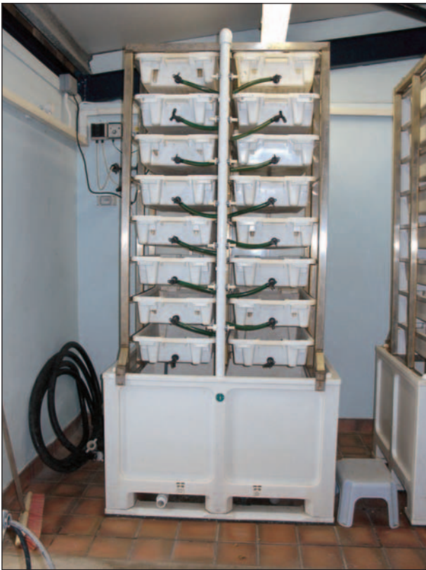
Figure 25. A vertical stack depuration system. The molluscs are held in purpose designed, solid sided containers which are either directly stacked or supported above one another in a frame over a sump tank. Seawater is drawn from the sump up to one end of the top container of the stack. It passes along the container and then cascades down from the other end into the container below and so on until it returns eventually to the sump.
