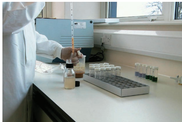
The E. coli analysis is being carried out showing the most-probable number (MPN) method.
