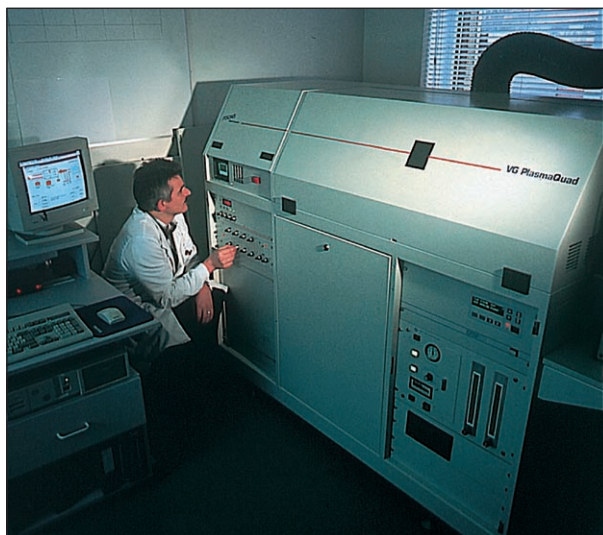
Figure 38. Inductively coupled plasma-mass spectrometry (ICP-MS) was used to analyse for certain metals.
