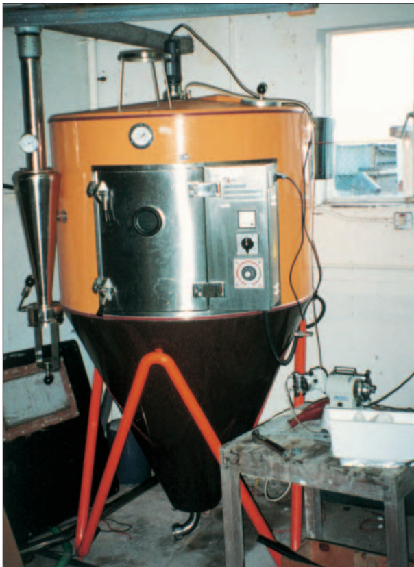
Figure 4. Preserving algae by spray-drying. The marine unicellular alga Tetraselmis suecica can be spray-dried to a powder. It can then be stored and re-hydrated as required for use as a supplement to feed bivalve mollusc juveniles.
