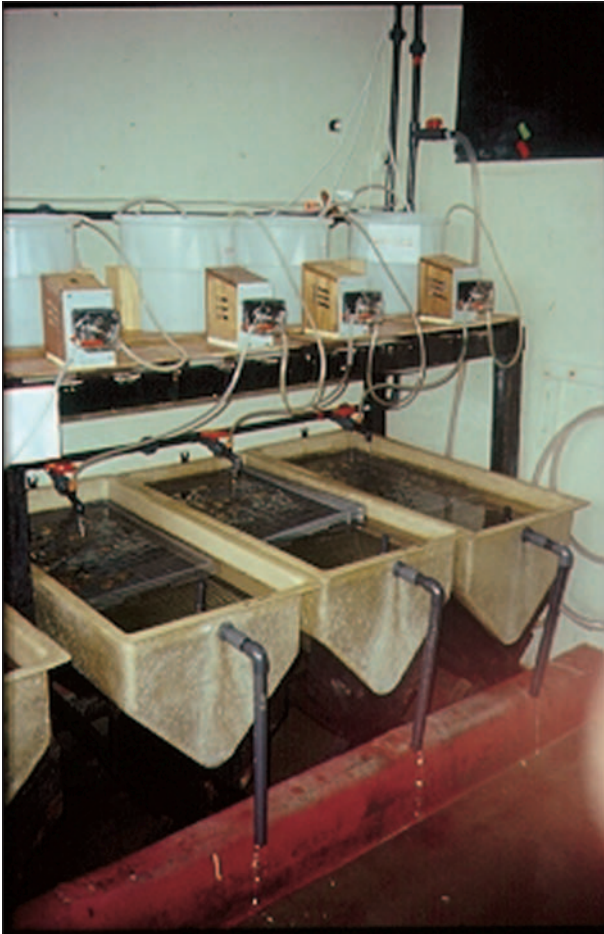
Figure 6. Broodstock conditioning experiments. Diet rations are metered into the seawater supply by the peristaltic pumps.
