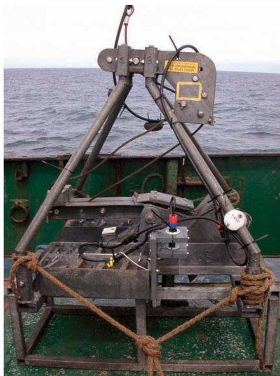
**Figure 3.1.** A 0.1 m<sup>2</sup> Hamon grab with attached video camera supported on an open frame to facilitate retrieval of the sample into a moveable container following controlled release from the grab bucket.
