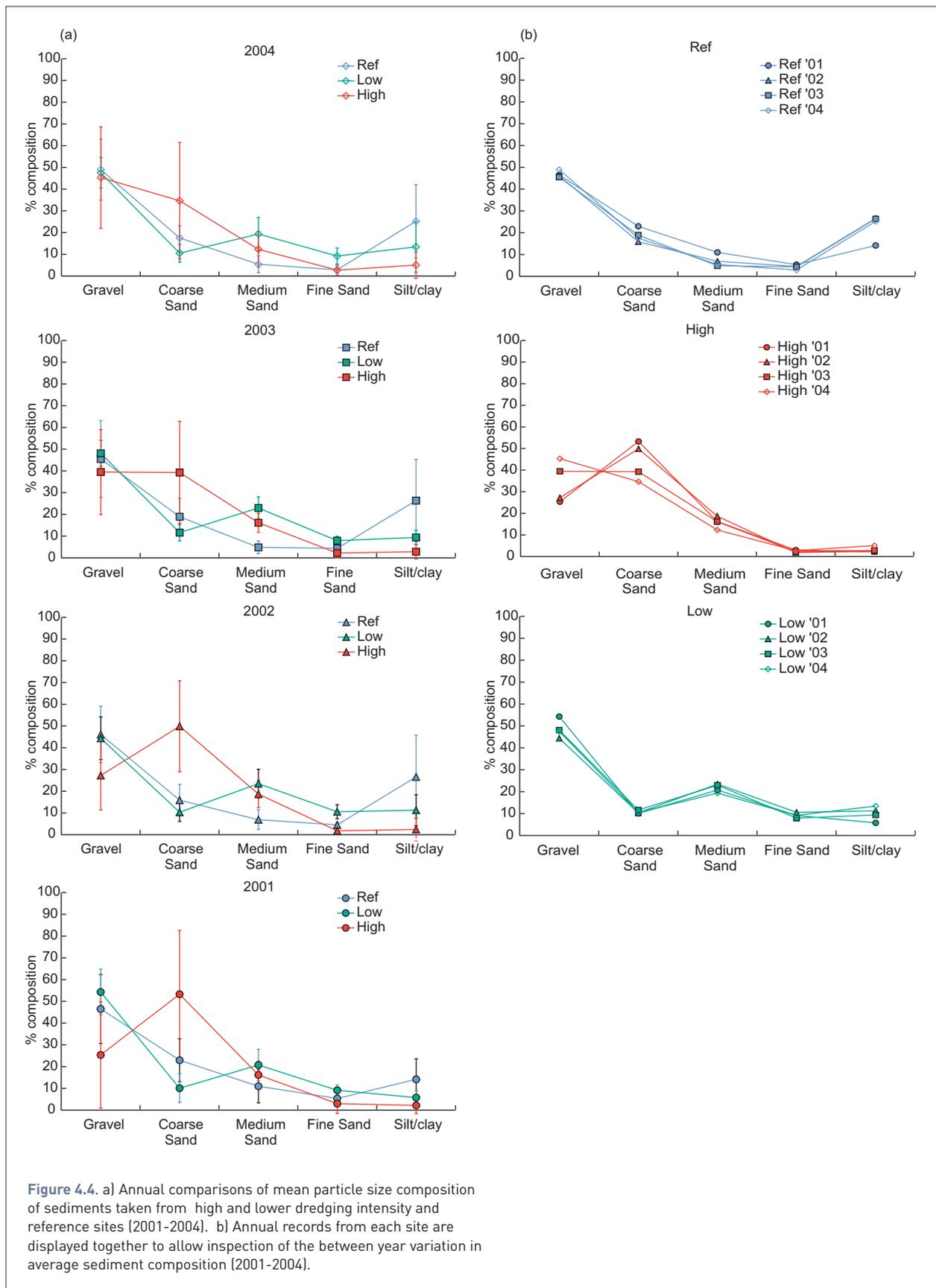
**Figure 4.4.** a) Annual comparisons of mean particle size composition of sediments taken from high and lower dredging intensity and reference sites (2001-2004). b) Annual records from each site are displayed together to allow inspection of the between year variation in average sediment composition (2001-2004).
