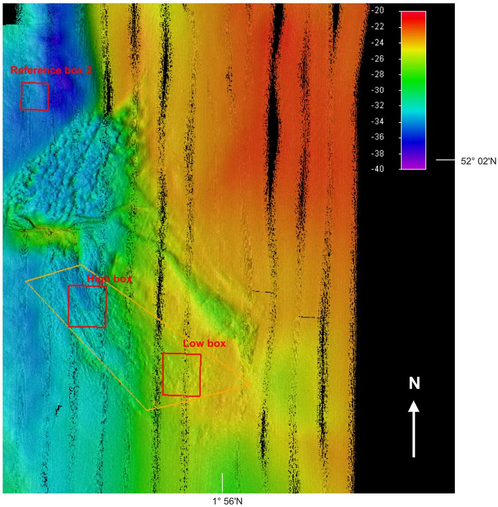
**Figure 4.9.** Overview of the Area 222 multibeam survey results from 2004. The orange line shows the outline of the former licensed extraction sites. Red boxes show the location of the study sites.
