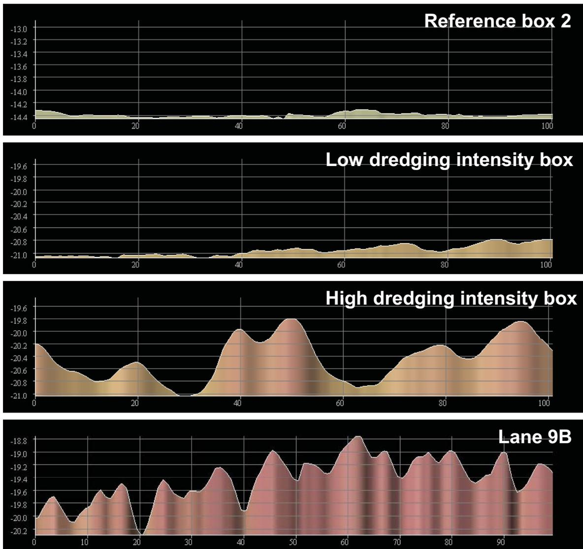
**Figure 5.18.** Seabed profiles from the 2003 multibeam bathymetric survey carried out at Hastings Area Y. The profile from lane 9B shows the impact of recent dredging activities.
