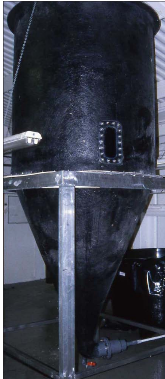
Figure 2.1. A 1150 litre tank for halibut yolk-sac larvae: the scale can be appreciated from the relative size of a fluorescent lamp unit suspended from the ceiling, and visible about halfway up the tank.
