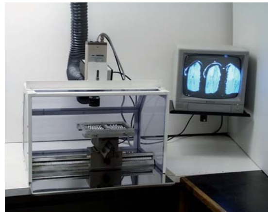
Figure 3. View of the mounting box showing the top mounted video camera, extractor vent to remove resin fumes and an alternative X-Y jig.
