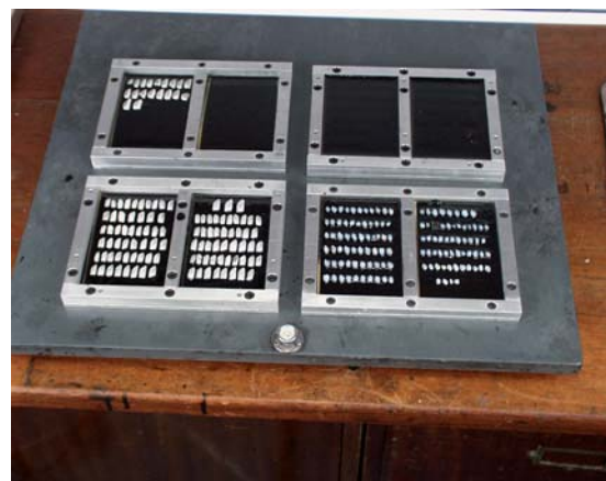
Figure 4. Otoliths of cod (left) and plaice (right) being added to moulds. The top right mould shows a completed mould after the top layer of black resin has been added over the otoliths.
