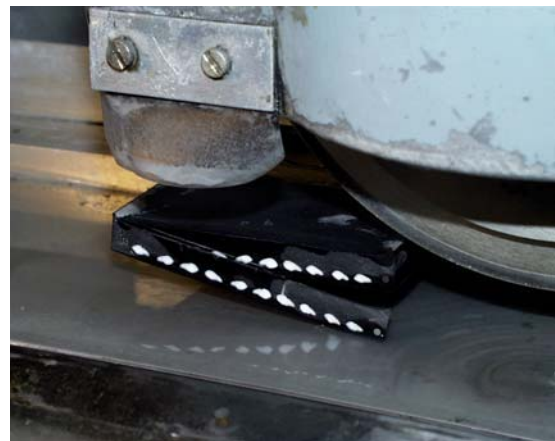
Figure 6. Cutting thin sections from the resin block using the Beacon cutter.
