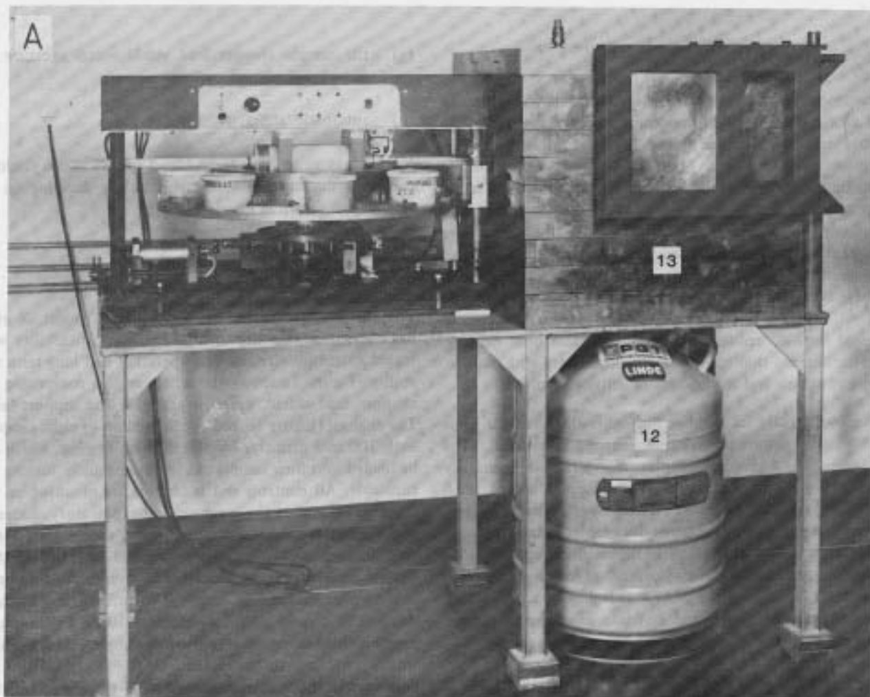
Figure 1 The sample changer system, with components identified by numbers: (a) overall view of the system comprising the changer (top left), lead shield (top right) and detector assembly (lower right) (b) The changer (c) The changer alone, with lead shield removed and position of detector head indicated.
