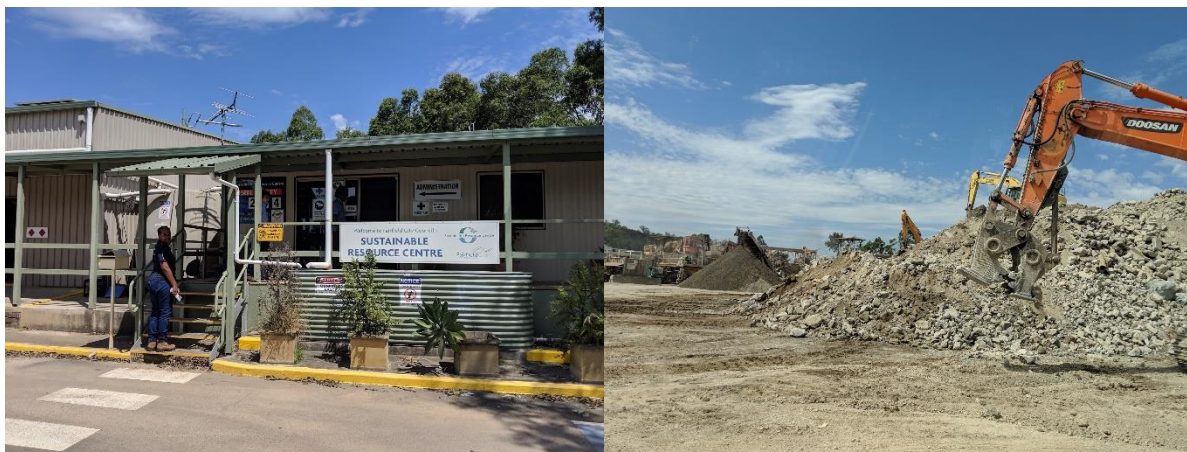
Image 11: Fairfield council concrete recycling facility. A jaw crusher attachment for an excavator is the most useful piece of equipment for concrete recycling
