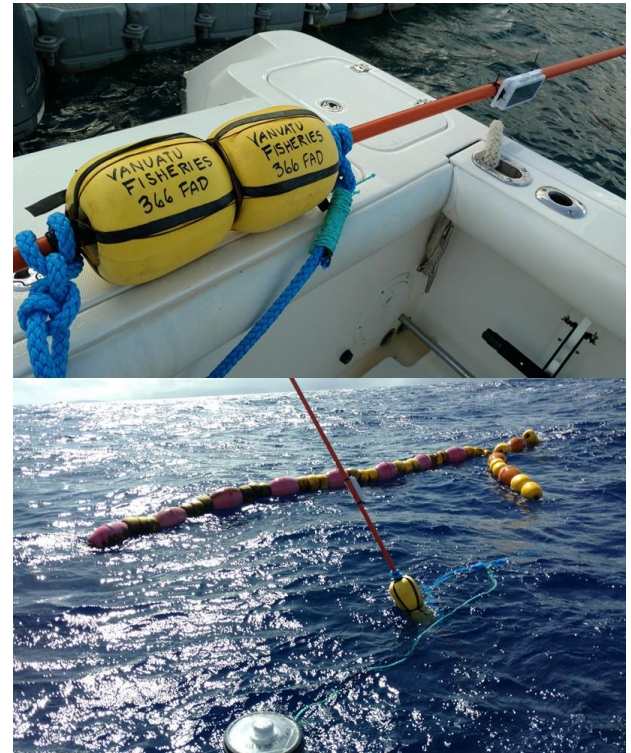
Figure 6. PDS unit and SatLink buoy attached to Vatuika AFAD.
