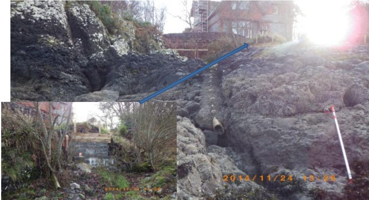
Figures 10 & 11 (insert). Two pipes from septic tank- samples taken from end of ceramic pipe and from plastic pipe associated with wp 15.
