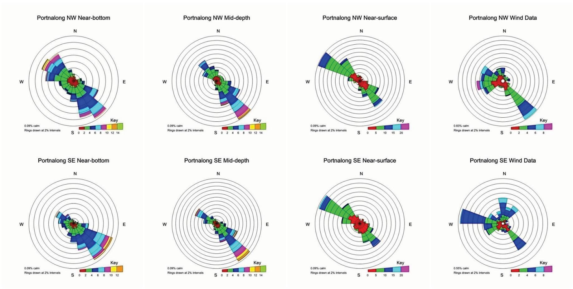
**Figure 14.5 Current and wind plots for the Portnalong NW and SE current meters**
