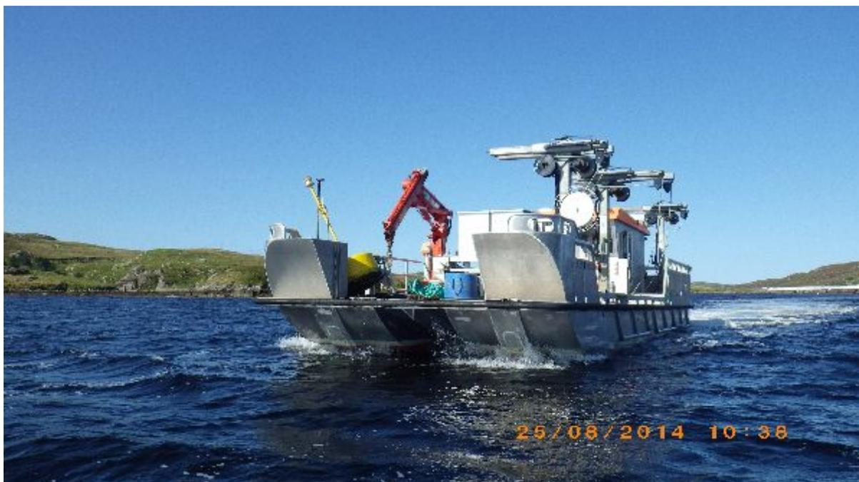
**Fig 6:** Aluminium mussel farm harvesting vessel – photo taken on passage in Loch Barraglom on return to shore base.
