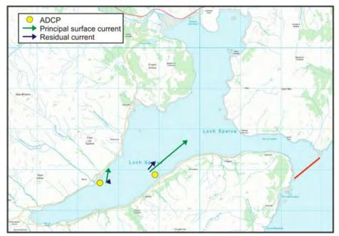
**Figure 13.4 Map showing Loch Spelve ADCP sample sites within the assessment area.** Using the surface principal current amplitude and residual current velocities and the assumption of a uniform sinusoidal tide, the cumulative transport distance and direction that might be expected during each phase of the tide is shown above.
