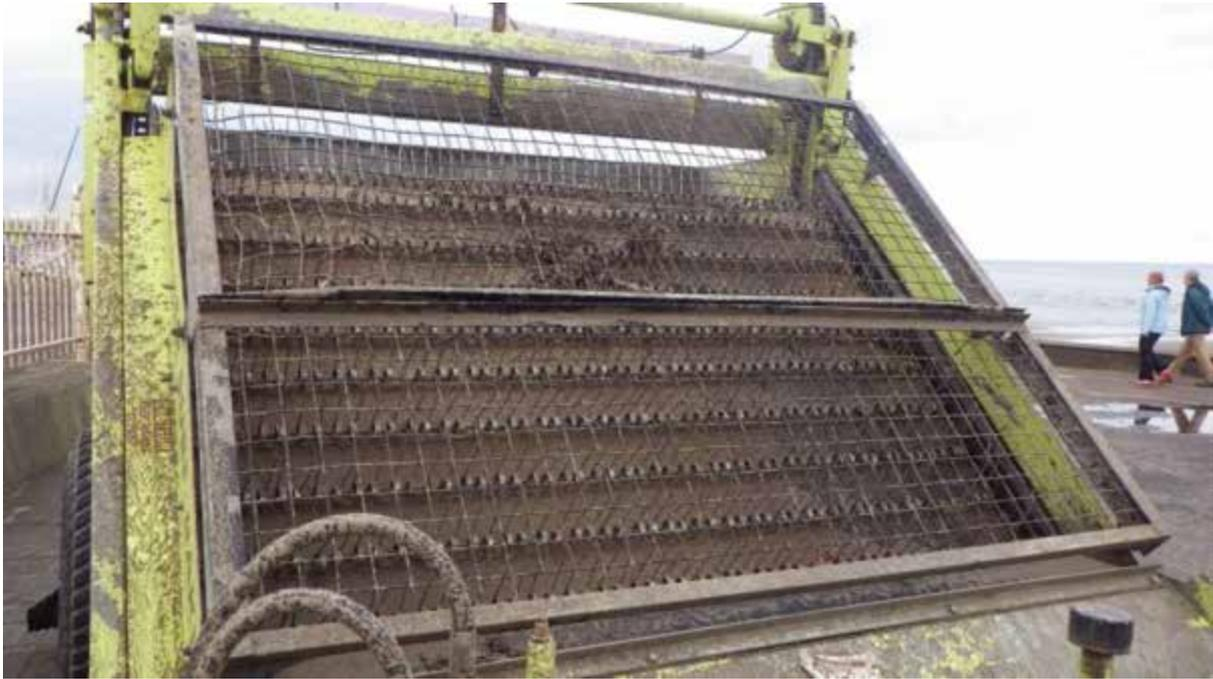
Figure 19 Tractor towed Barber Surf Rake operated by South Ayr Council beside Prestwick Sailing Club. Near to Waypoint 57.
