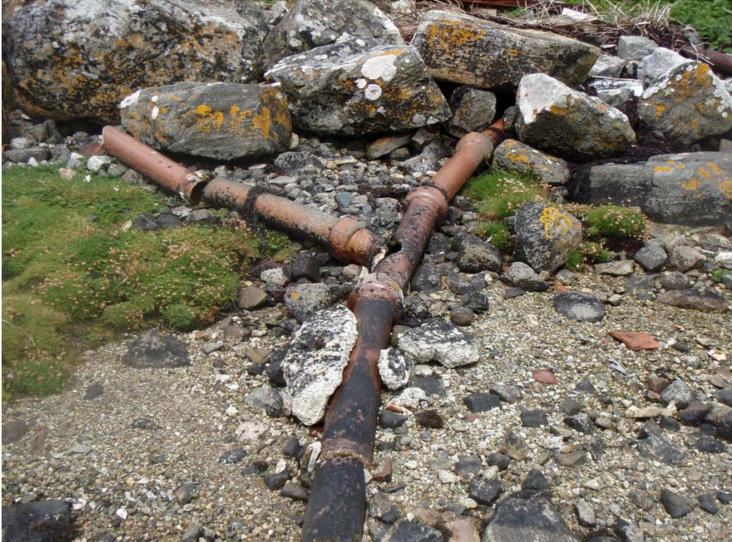
Figure 16. Broken pipe, no flow
