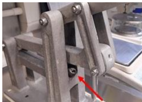
Figure 3: Opening a gastropod using an oyster cracker
