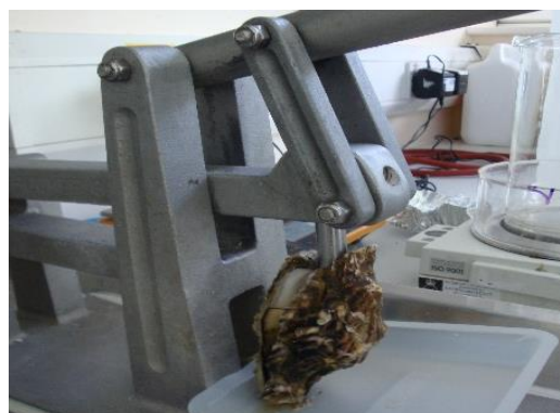
Figure 2: Opening an oyster using an oyster cracker
