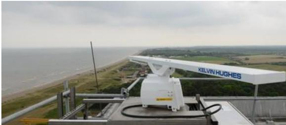
Coastal marine conditions, including wave parameters and surface current velocities, can be measured using a standard marine X-Band radar and specially developed software. Spatial resolution and range are variables determined by the nature of the instrument's installation and project requirements.
