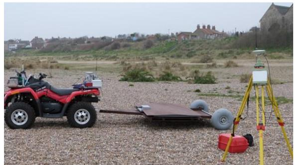
Using a towed receiver, sediment transport surveys can be quickly undertaken, highlighting the mobility regimes in place for specific sediment types/sizes.
