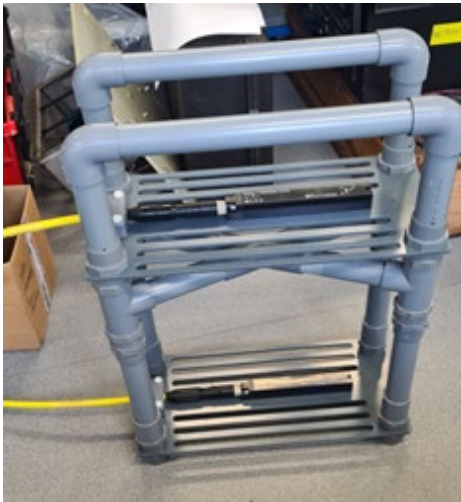
Figure 8(a) Magnetometer set up used for field surveys. Black magnetometers were set up in the same horizontal orientation but were separated 0.5 m vertically. Yellow 20 m cables from the magnetometers were attached to (b) The Spectramag-6 Data Acquisition Unit which was linked to a laptop with the Spectramag-6 software.
