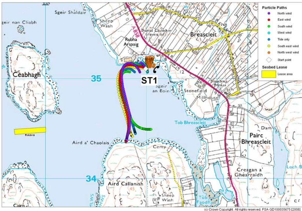
Figure 13.4 a: particles paths of particles released at sources ST1. Particles released at every hour and under different wind directions (no wind, north, east, south, west, northwest and southeast winds).
