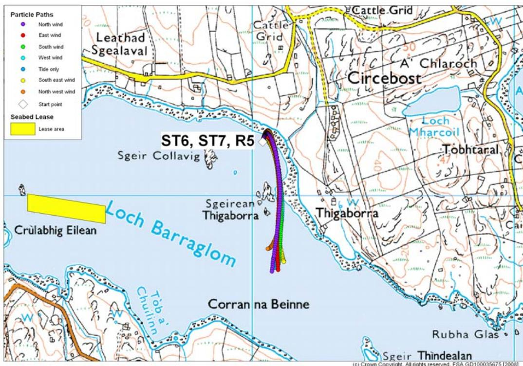
Figure 13.4 g: particles paths of particles released at sources ST6, ST7 and R5. Particles released at every hour and under different wind directions (no wind, north, east, south, west, northwest and southeast winds).
