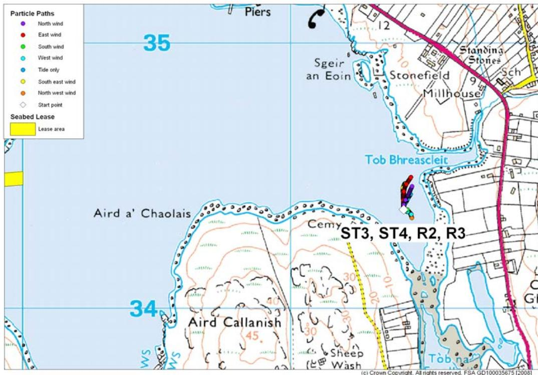
Figure 13.4 c: particles paths of particles released at sources ST3, ST4 and R2, R3. Particles released at every hour and under different wind directions (no wind, north, east, south, west, northwest and southeast winds).
