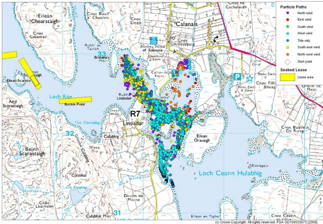
Figure 13.4 f: particles paths of particles released at source R7. Particles released at every hour and under different wind directions (no wind, north, east, south, west, northwest and southeast winds).
