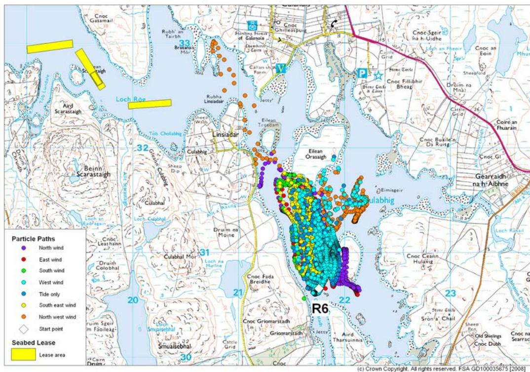
Figure 13.4 e: particles paths of particles released at source R6 (Grimersta river). Particles released at every hour and under different wind directions (no wind, north, east, south, west, northwest and southeast winds).
