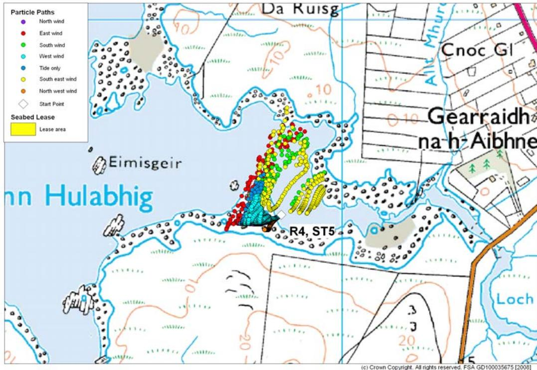
Figure 13.4 d: particles paths of particles released at sources ST5 and R4. Particles released at every hour and under different wind directions (no wind, north, east, south, west, northwest and southeast winds).
