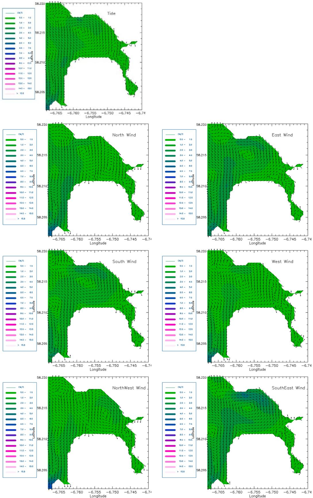
Figure 13.5: Residual currents in Breasclote Bay for tidal forcing only and with imposed wind directions. Colour distribution indicates residual current speed and arrows give the direction. Arrows plotted at every model grid point.
