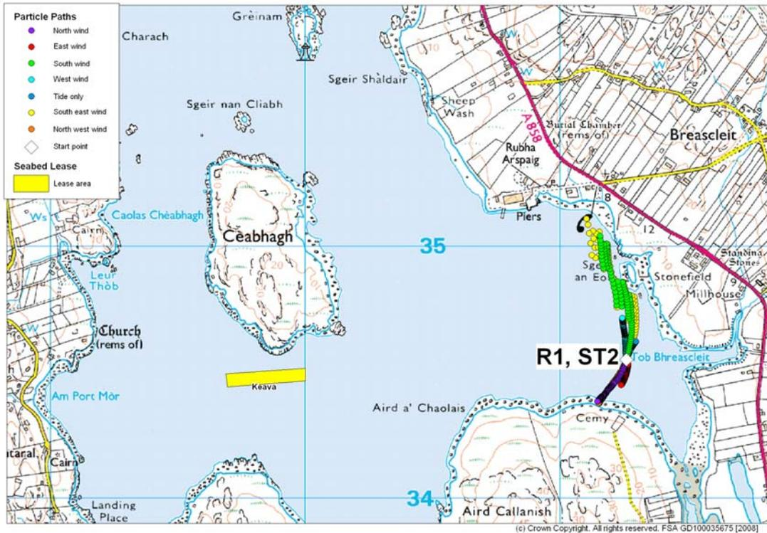
Figure 13.4 b: particles paths of particles released at sources ST2 and R1. Particles released at every hour and under different wind directions (no wind, north, east, south, west, northwest and southeast winds).
