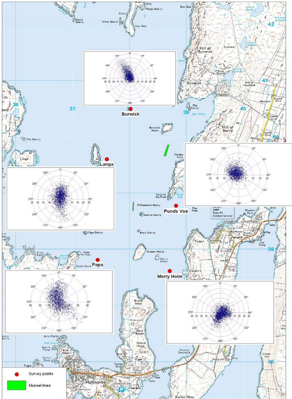
Figure 13.4 Polar plots of tidal direction and velocity readings near the surface for the five fish farm study sites.
