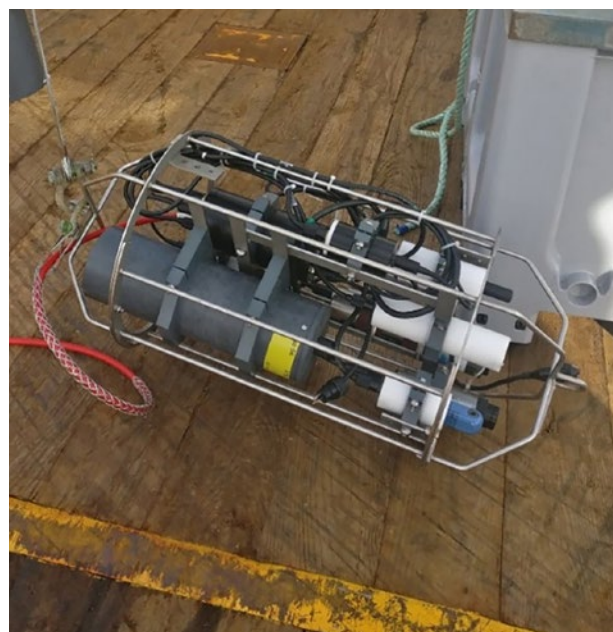
Figure 3: Multi-Sensor Logging Platform data logger with pressure, temperature, and conductivity sensors, in addition to a PAH sensor and a turbidity sensor.
