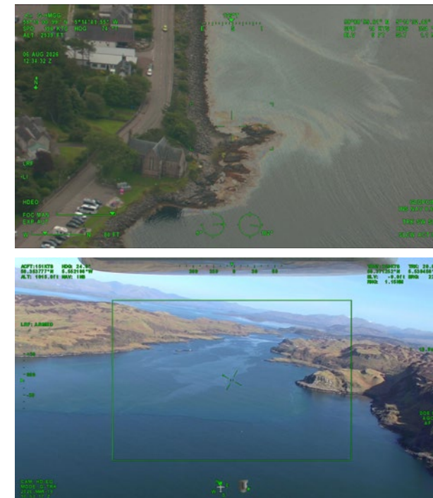
Figure 12: Examples of aerial surveillance imagery used to identify, quantify and monitor marine pollution, including oil contamination in coastal and nearshore environments © Maritime and Coastguard Agency (MCA).
