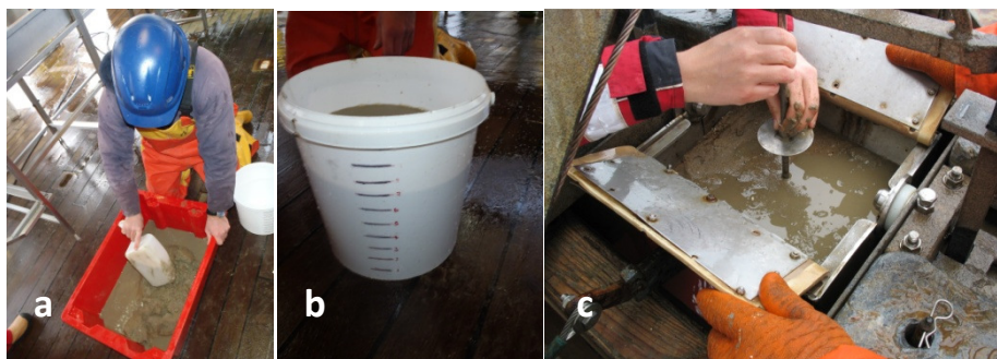
Figure 9. Measuring the volume of a Hamon grab sample (a-b) and depth of a Day grab sample (c)
