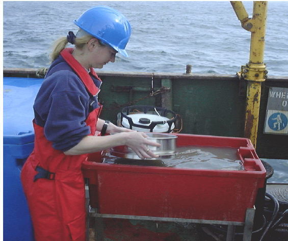
Figure 12. Puddling the sample to remove the fine sediment fraction
