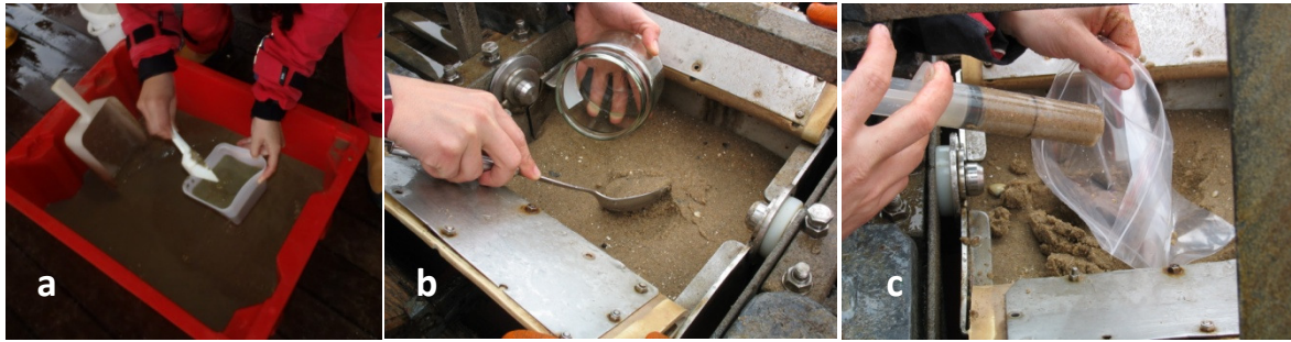
Figure 7. Taking relevant sedimentary subsamples for further contaminants and particle size analysis (a, Hamon grab, b-c, Day grab)
