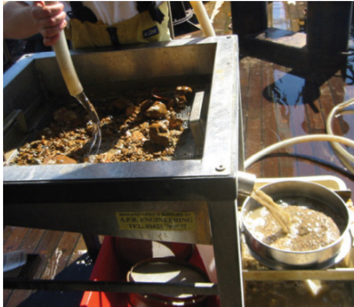
Figure 10. Washing the sediment sample through a 5 mm top sieve mesh into a 1mm sieve mesh.
