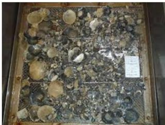
Figure 11. An example photograph of sediment retained on the 5mm sieve mesh
