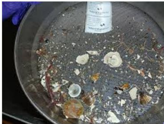
Figure 13. An example photograph of sediment retained on the 1mm sieve mesh
