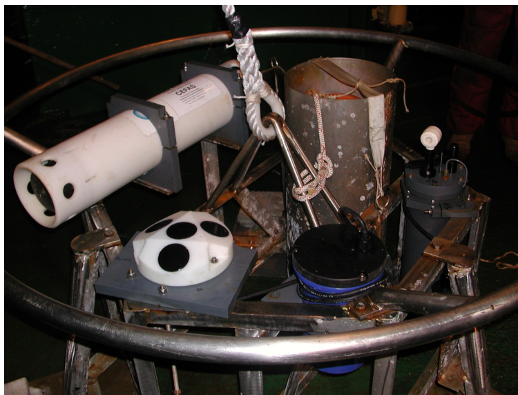
Figure 4 - Seabed frame with Acoustic Current Meter and water quality instruments.
