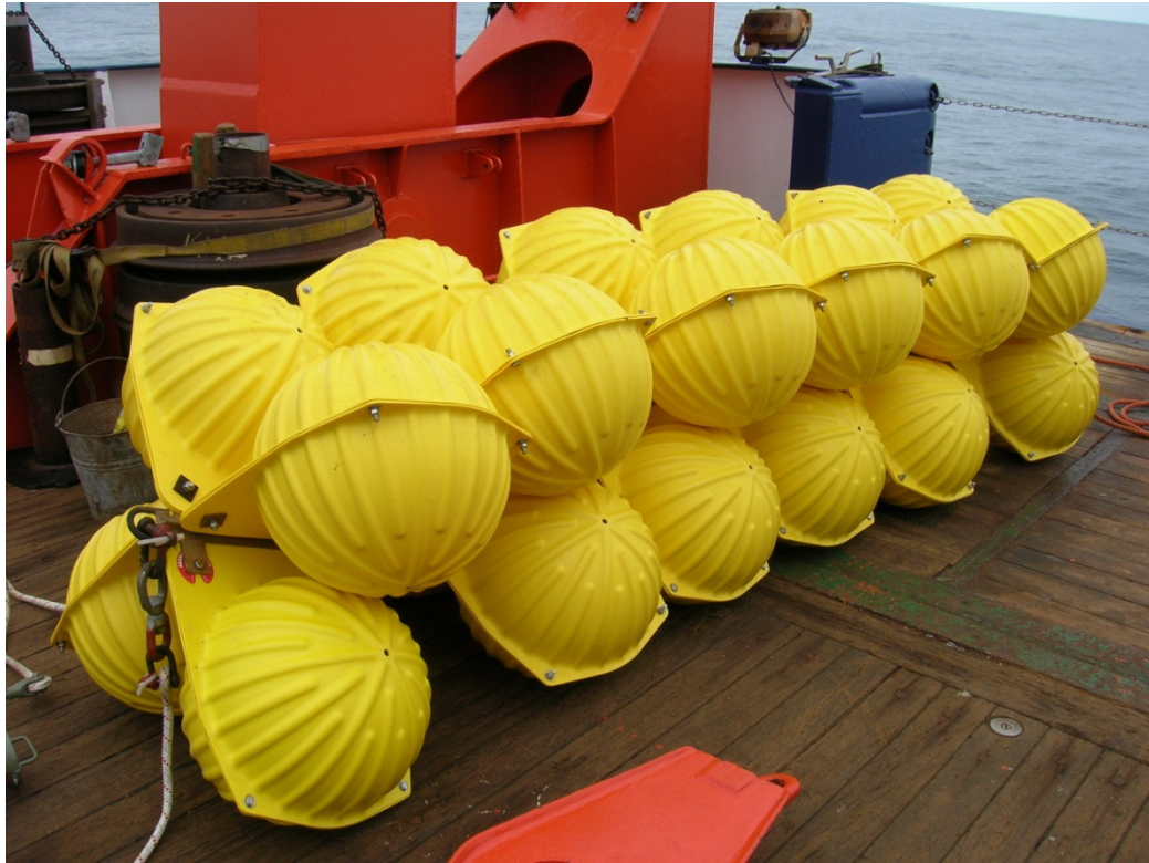
Figure 1 - Glass Sphere Buoyancy for moorings.
