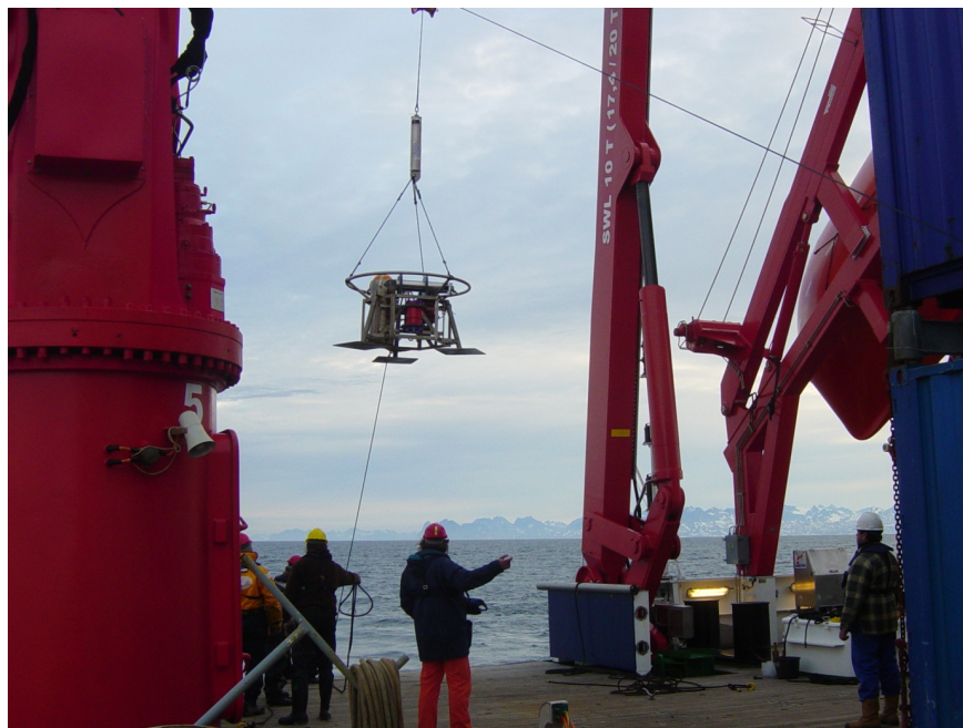
Figure 3 - Preparation to deploy a seabed mounted upward looking Acoustic Current meter.
