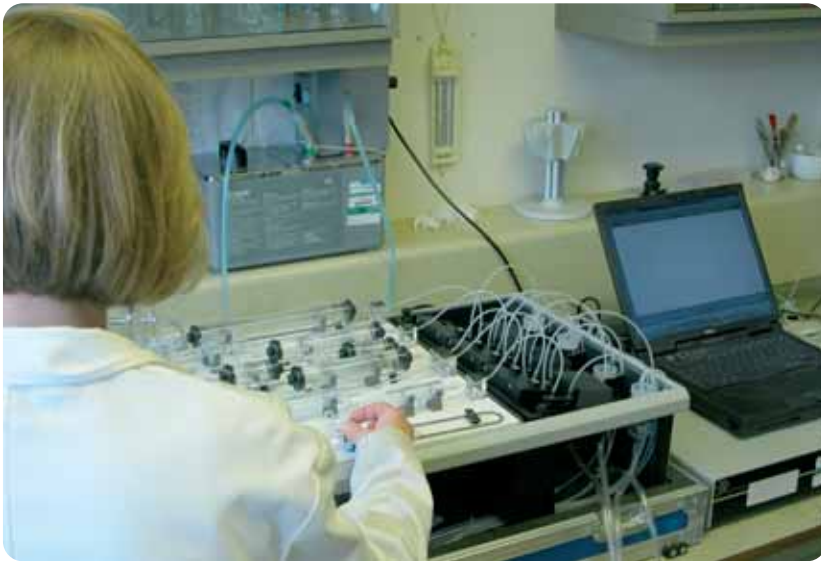
Above: Auto-analyser used to analyse water samples collected using CTD Rosette or Aquamonitor
