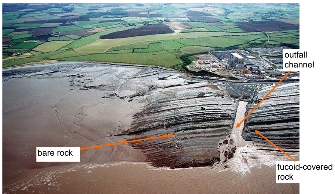
Figure 28 Hinkley Point outfall channel from the air, showing seaward-facing limestone slopes colonized by fucoid algae (dark areas)
