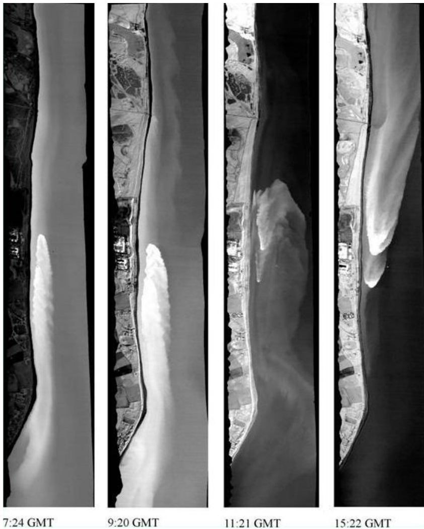
Figure 6 Outfall plume of Sizewell A&B Power Station showing flood tide (7:24 GMT and 9:20 GMT); slack water (11:21 GMT); and ebb tide (15:22 GMT) (source: Environment Agency)
