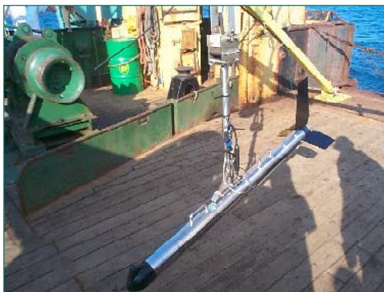
Figure 28 Datasonics™ SIS 1500 Chirp sidescan sonar fish. This device acts as a stable platform for the transducers, and is towed behind the vessel during the survey
