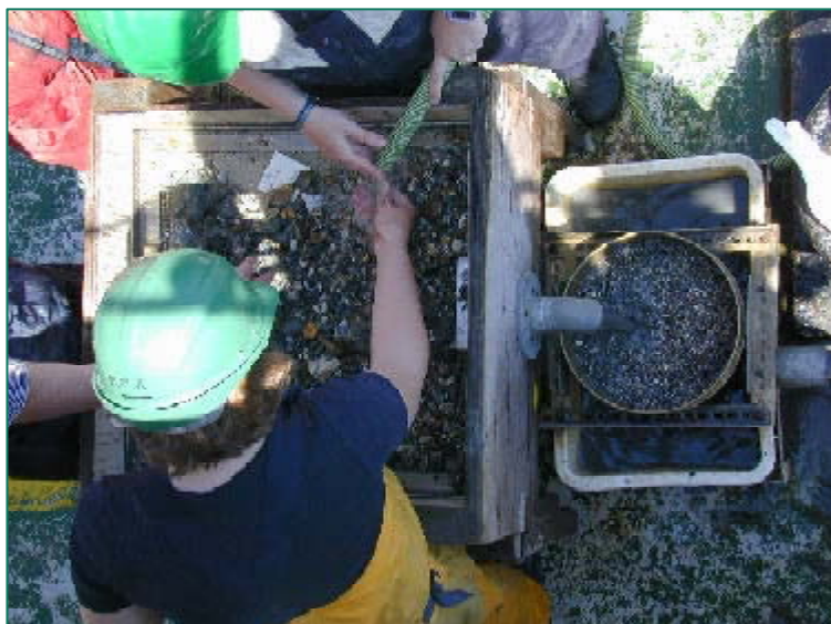
Figure 19 Processing of a macrofaunal sample using a purpose built sieving table on a survey vessel. The sample is being washed over a 5 mm square mesh aperture sieve supported by a removable square stainless steel frame. Note also the 1mm mesh sieve held within a sieve holder beneath the outlet pipe of the table
