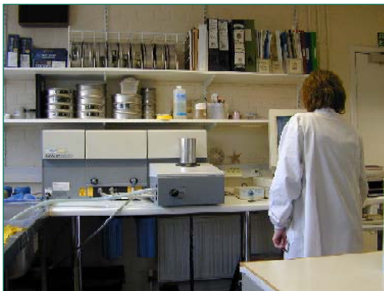
Figure 35 Coulter™ LS 130 laser sizer. This equipment uses laser diffraction technology to measure particle diameters. It is most frequently used to measure the finer component (<500 µm/<63 µm) of a sediment sample
