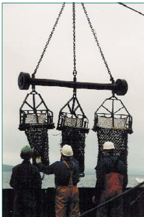
Figure 12 A Newhaven Scallop dredge. Note the robust metal beam with rubber rollers on each end. Three dredges are attached to the beam, and the upper nylon mesh side of the collection bags are visible
