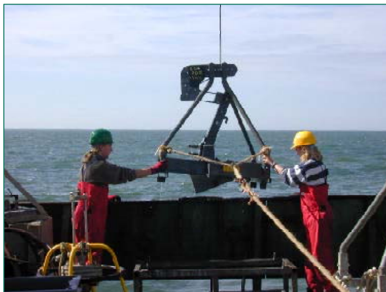
Figure 6 A 0.1 m 2 Hamon Grab being retrieved. Note the use of a winch-controlled lateral supporting rope for increased stability (and therefore safety) during deployment and recovery. It is unhooked before descent of the sampler
