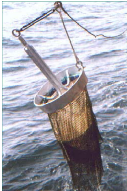
Figure 13 A Raillier-du-Baty dredge. The dredge consists of a robust circular metal mouth to which a collection bag is attached. The dredge is towed from the bridle attached to the outer rim of the dredge. A weak link between the towing bridle and the central towing arm of the dredge is designed to break if the dredge meets an obstruction on the seabed
