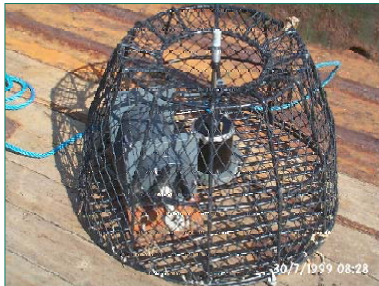
Figure 32 CEFAS loggerpot which contains an ESM2 burst logger recording suspended sediment concentration, tidal elevation, wave statistics, conductivity and temperature. Also mounted in the Loggerpot is a Falmouth Scientific Instrument 2D Acoustic Current Meter (ACM)
