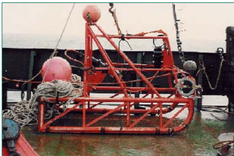
Figure 16 A CEFAS camera sledge. Note the downward pointing 35 mm stills camera at the front of the sledge and the forward looking video camera towards the rear of the sledge. The large buoy on the back of the sledge floats at the surface during deployment, and provides a visual indication of the position of the sledge. It also acts as a means of recovery for the main towing cable parts
