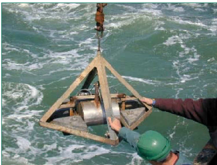
Figure 8 A 0.1 m 2 Day grab during deployment. Note that the sample buckets are in the open position prior to sampling. Also note the addition of triangular lead weights to improve sampling efficiency
