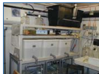
Figure 4: Photograph of the flow-through system set-up in a constant temperature room (14 ± 1 °C) at CEFAS Burnham laboratory.
