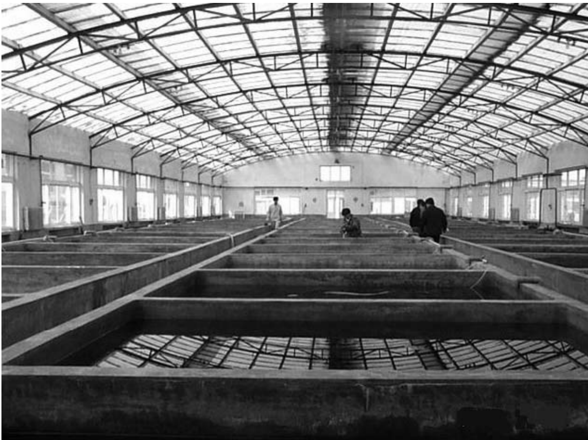
Large land based cement tanks are used for broodstock conditioning, microalgae production, larvae culture and early juvenile nursery
