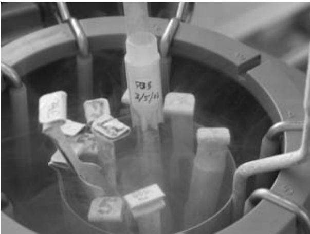
Cryovials are used to store sperm
