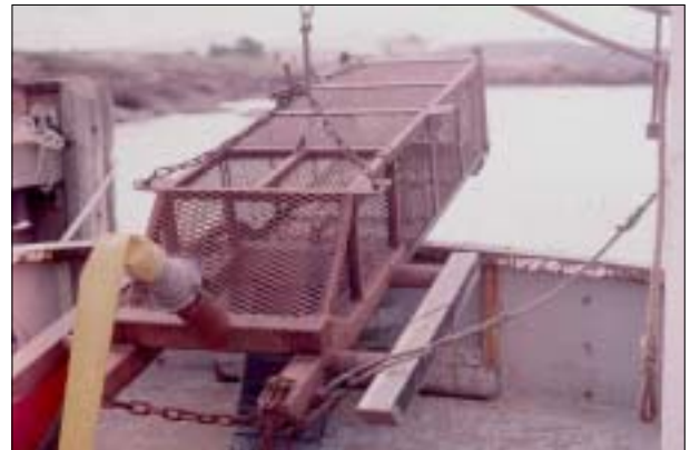
A toothed hydraulic dredge used to fish the razor clam Ensis spp.
