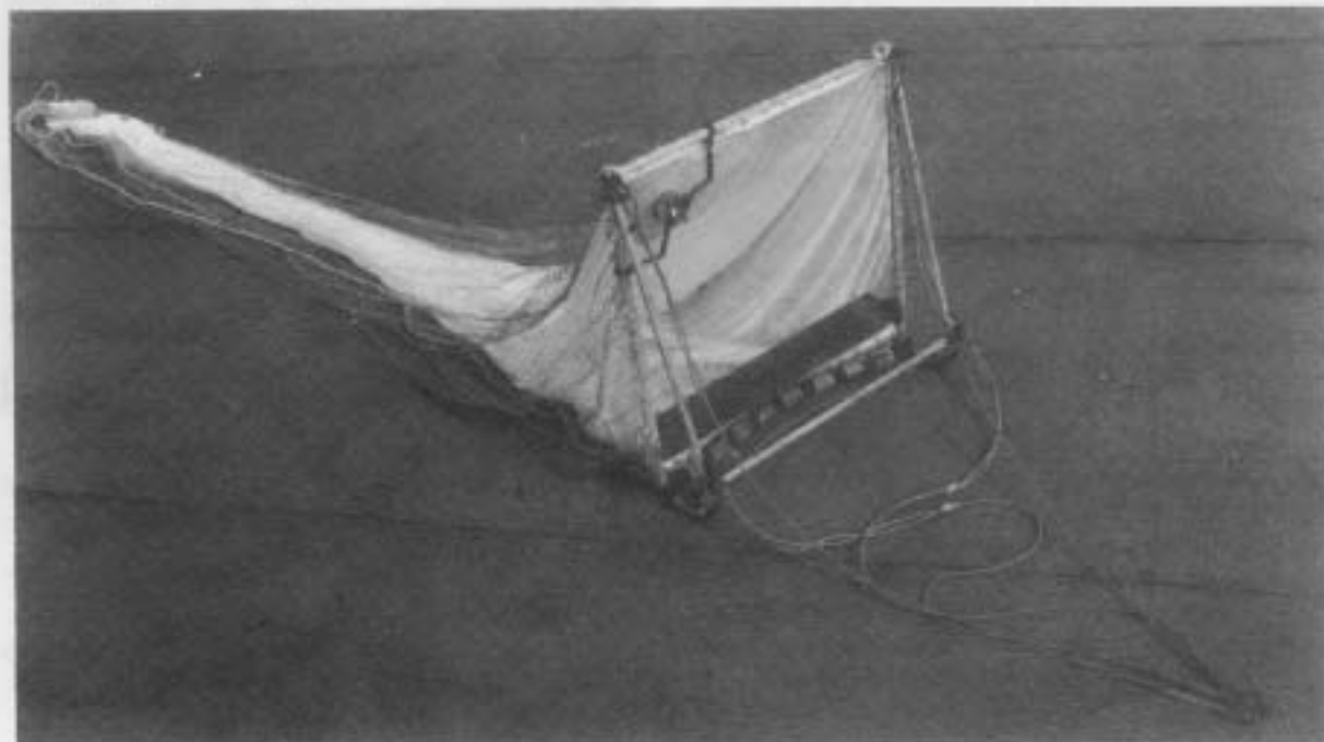
Figure 1 The 2 m 2 frame trawl.
