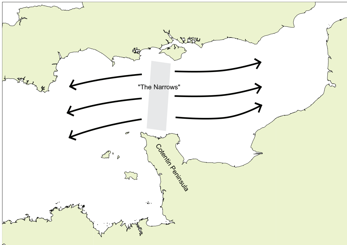
Figure 4: Schematic representation of the bedload parting zone and net transport directions in the central English Channel. (after Hamblin et al , 1992)
