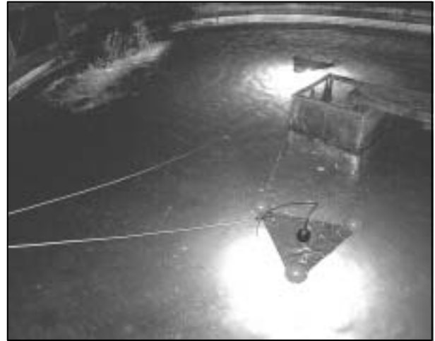
Figure 3. Floating light units used to provide artificial illumination in outdoor ponds
